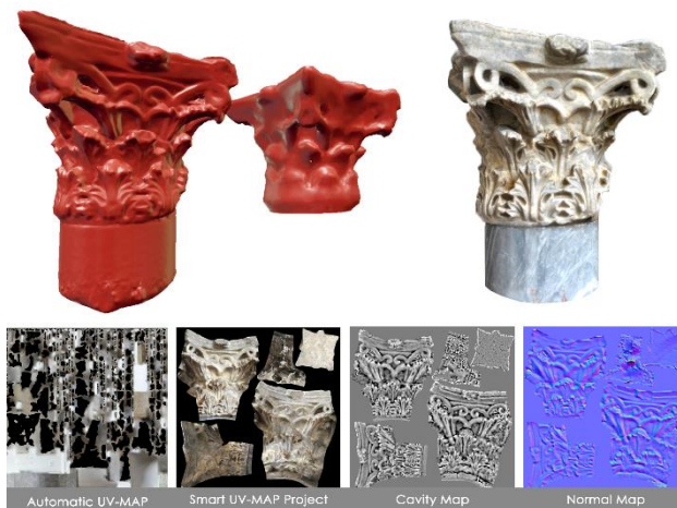
Figure 3. The Retopology phase on an architectural element and the Baking one by procedural 2D maps
