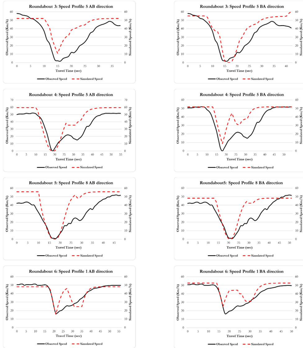
Figure 4.5: Observed speed-time profiles (reference) vs (default) simulated speed profiles for the roundabouts sample
