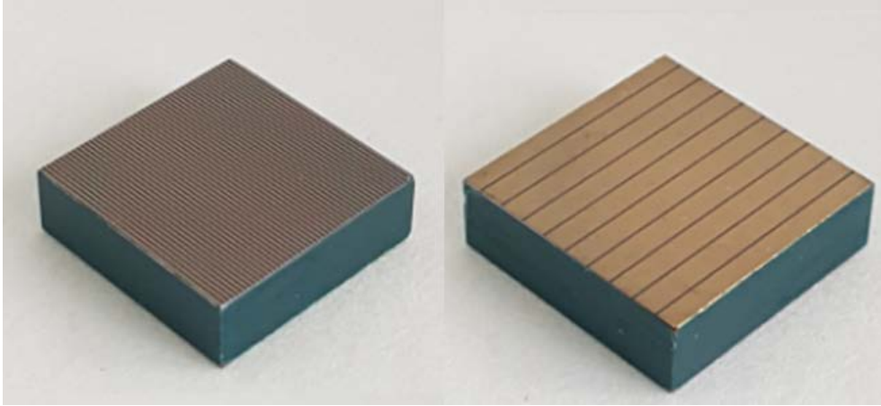
Figure 3.3 Anode (left) and the cathode (right) layouts of the CZT drift strip detectors. The anode strips (0.4 mm pitch; 0.25 mm gap) are orthogonal to the cathode strips (2 mm pitch; 0.1 mm gap). The anode strips are organized into collecting strips (1.6 mm pitch) and drift strips (0.4 mm pitch) which are negatively biased to optimize electron charge collection.
