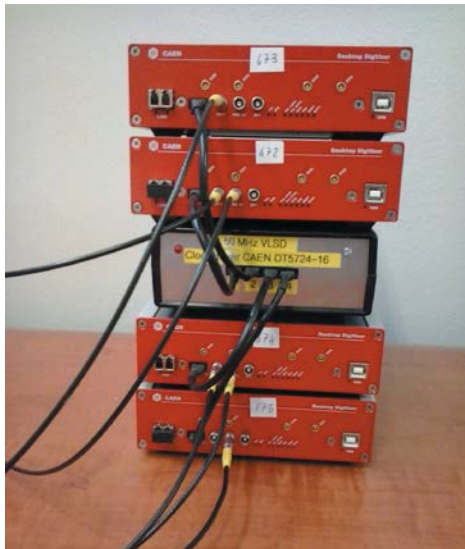
Figure 2.5 The 16-channel digital readout electronics. The central box is the clock splitter used to synchronize all digitizers.
