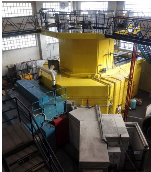
Figure 3.7 The TRIGA Mark II Reactor at L.E.N.A. of the University (Pavia, Italy).
