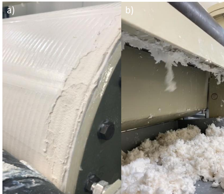
Figure 7. a) Magnesium cake on the filter cloth surface and b) detached magnesium hydroxide in the collection tray.
