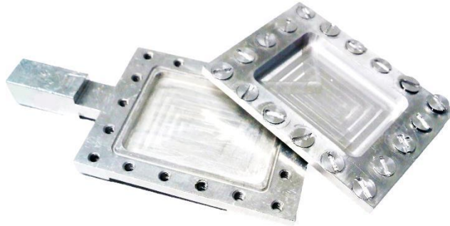
Figure 19. 600 \mu\text{l} opened sample cell for neutron scattering experiment consisting of a pan with indium fiber along its perimeter and lid with screws.
