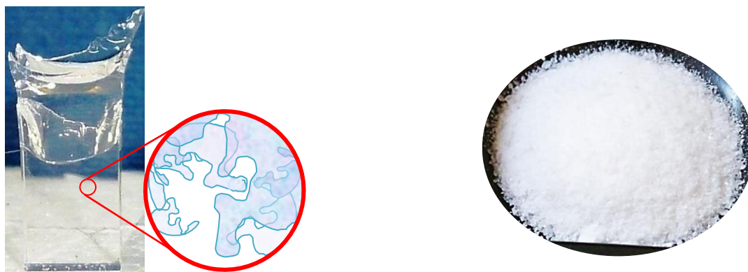
Figure 28. Left panel: solid 3D-disordered SiO 2 matrix with water in its pores and schematic representation of microscopic view inside of it (pores with water by blue and empty space by white). Right panel: silica powder obtained after crunch of solid matrix from left panel.
