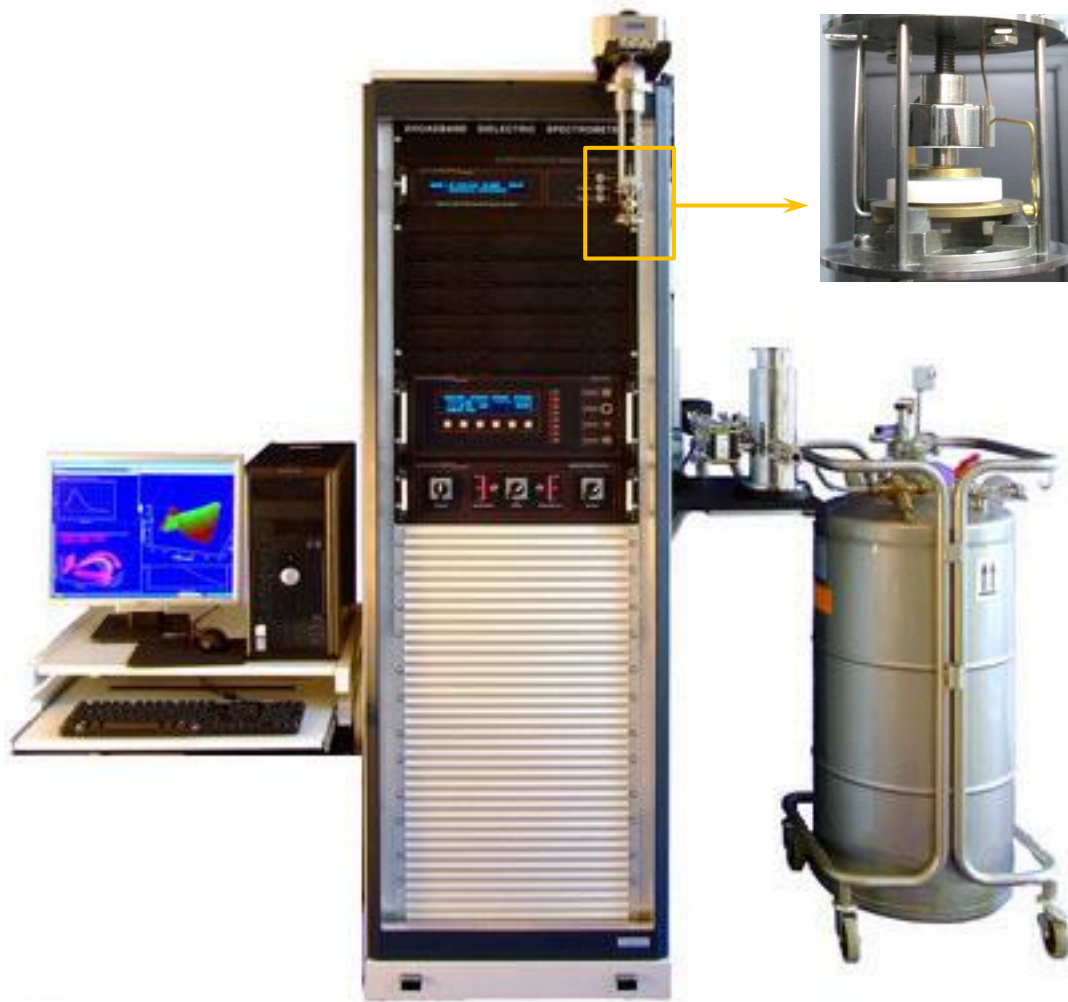
Figure 8. Alpha-A High Resolution Broadband Dielectric Spectrometer (Novocontrol, Germany) that was used to carry out all dielectric measurements.
