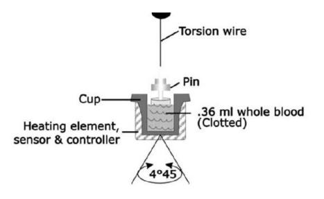
A depiction of a TEG device in which a pin suspended from a torsion wire is immersed in a cup of whole blood. The cup is held in a heating block and continually oscillates through 4\_450 every 5 sec. Changes in viscoelastic clot strength are directly transmitted to the torsion wire and detected by an electromechanical transducer. (Adapted from TEG and ROTEM: technology and clinical applications Am J Hematol . 2014 Feb;89(2):228-32.)
