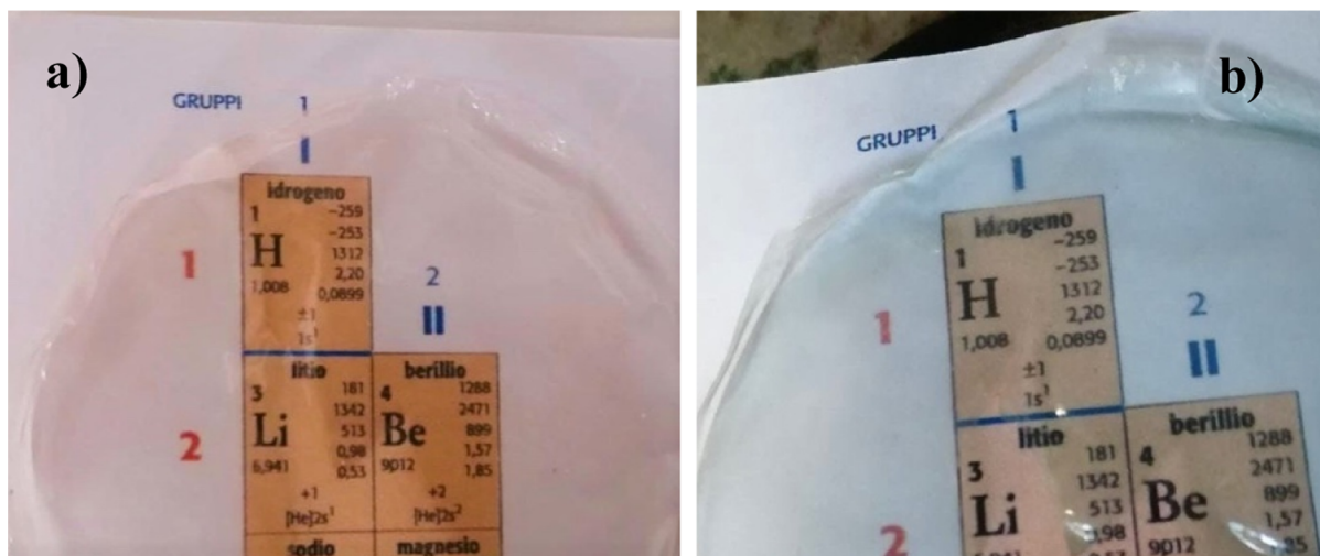
Figure 7. Thermochromic polymeric film [N_{1.1}3GA_8]Br/Co(NTf_2)_2/PMMA (3:1) (390 mg): (a) 25; (b) 80 °C.
