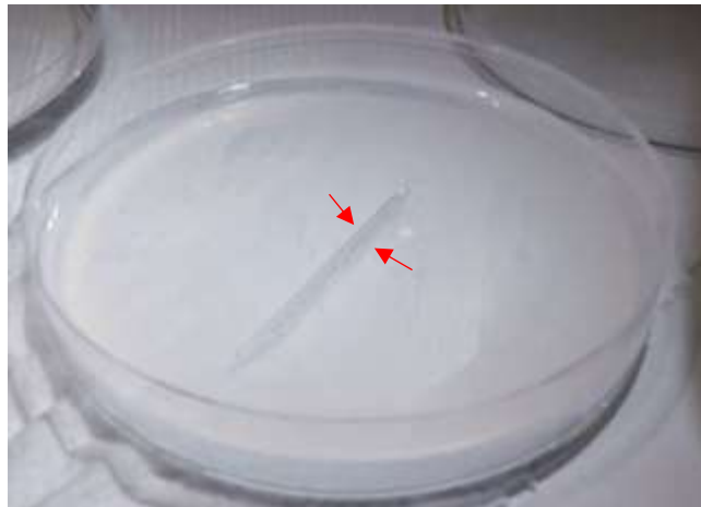
Figure 1. Handcrafted larvae holder. Red arrows point at the capillaries creating the support for larvae.
