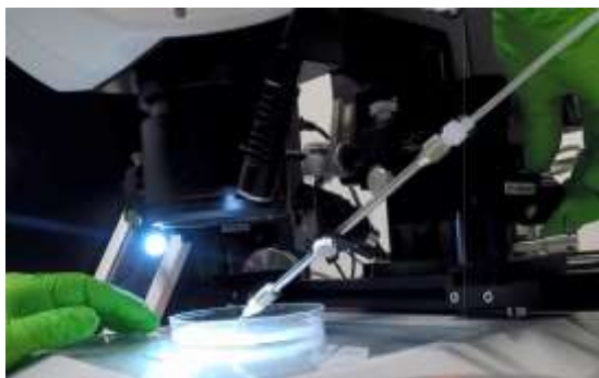
Figure 3. Preparing the microinjection apparatus under the stereomicroscope before starting session.
