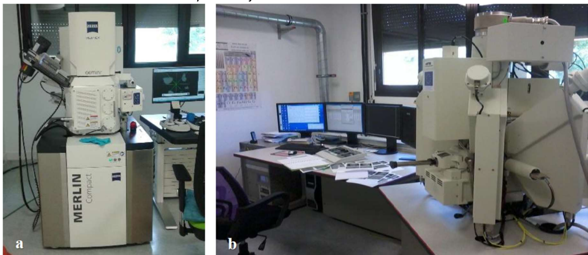
Fig. 15. a) Scanning electron microscope and b) electron microprobe at the ISTO. These two instruments were used for observation and analysis of major elements of the olivine and hosted MIs.
