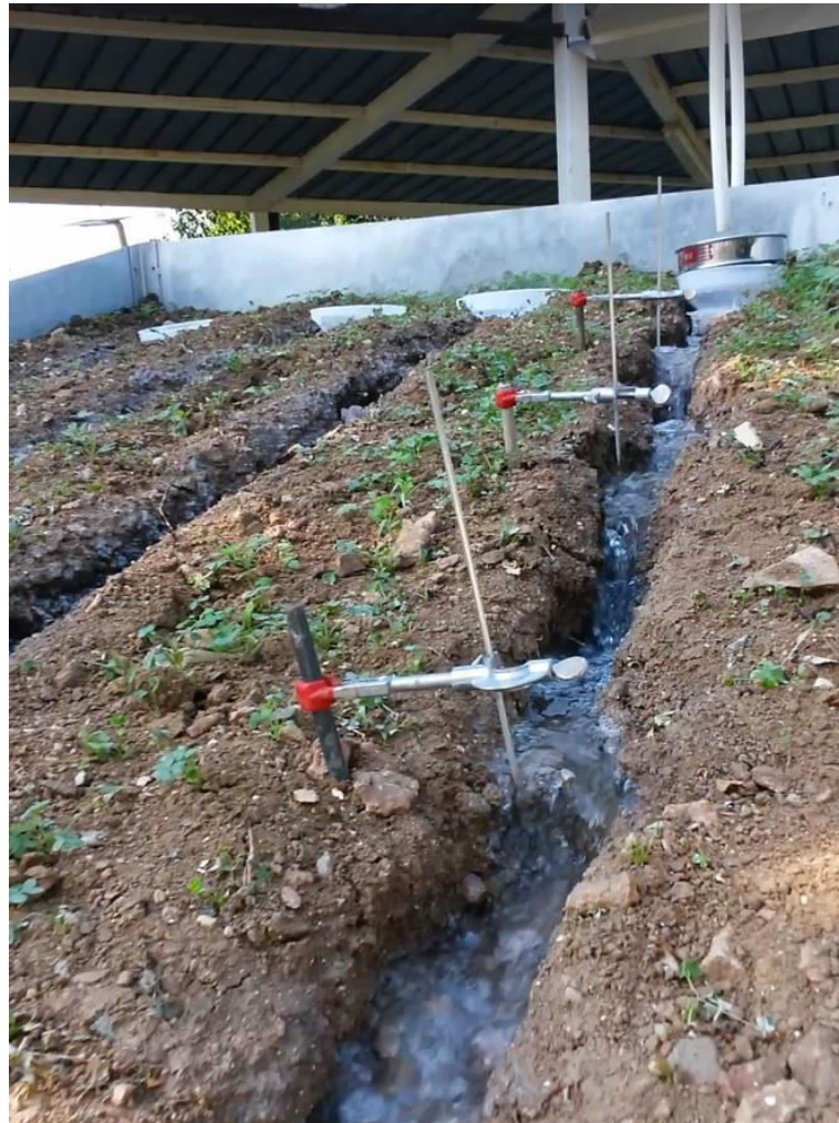
Figure 6. View of a step-pool sequence occurred during an experimental run.
