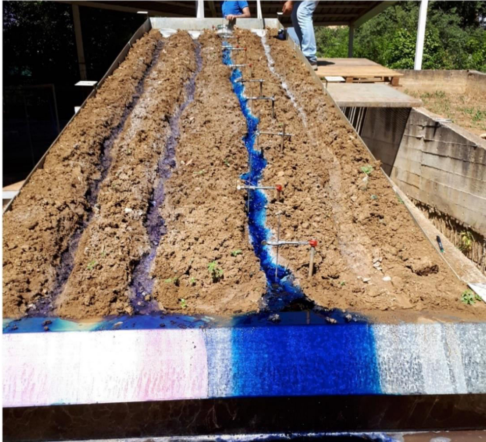
Figure 18. Flow velocity measurement by the dye tracing method using a Methylene blue solution.
