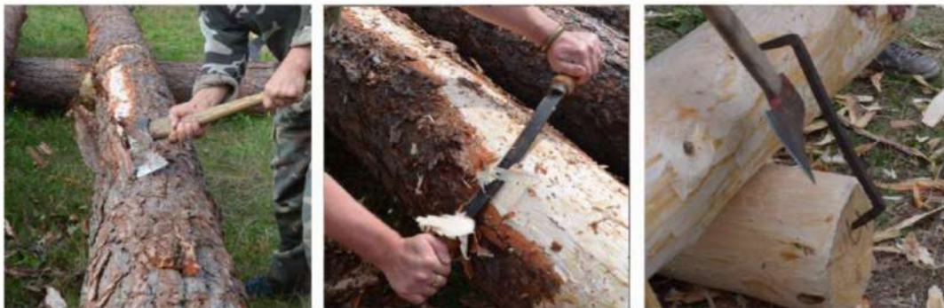
Fig. 4: Tools for debarking (a,b), vise tool for consolidation of logs.
