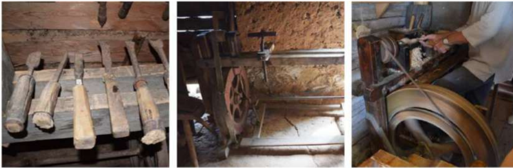
Fig. 6: Tools for turning and planing (a), lathe (b), turning (c).
