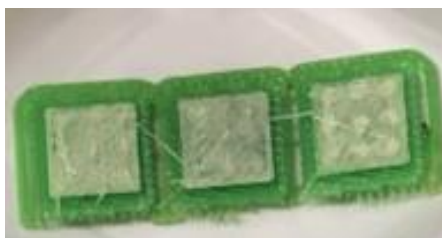
Figure 55. 3D printed patch 1cm 2 printed with 65% infill. Each printing allows obtaining from three to nine samples per time, representing a good advantage in scalability.
