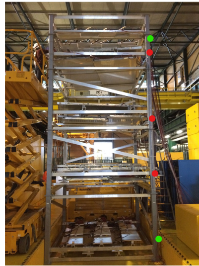
Fig. 1. (a) 3D model of the MATHUSLA test stand. (b) Photo of the final assembled structure installed above the ATLAS IP. The green dots identify the two scintillator layers used for triggering, while the red dots mark the three RPC double-layers used for tracking. (For interpretation of the references to color in this figure legend, the reader is referred to the web version of this article.)
