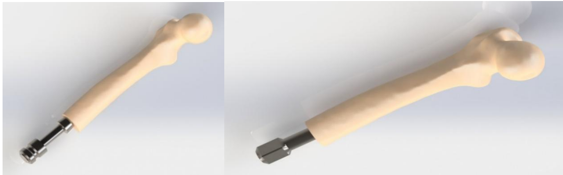
Figure 6. CAD models of the implant/bone assemblies: OPL (on the left) and OPRA (on the right).
