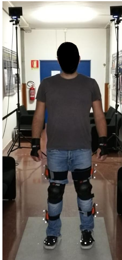
Figure 3. Subject equipped with protections and reflective markers for motion capture.
