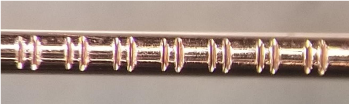
Figure 3.23. Picture, taken via an optical microscope, of the sample featuring the multiscale trenches, the procedure of which is shown in Figure 3.13. Note that, at this scale, the sample shows a good uniformity in the structure periodicity.
