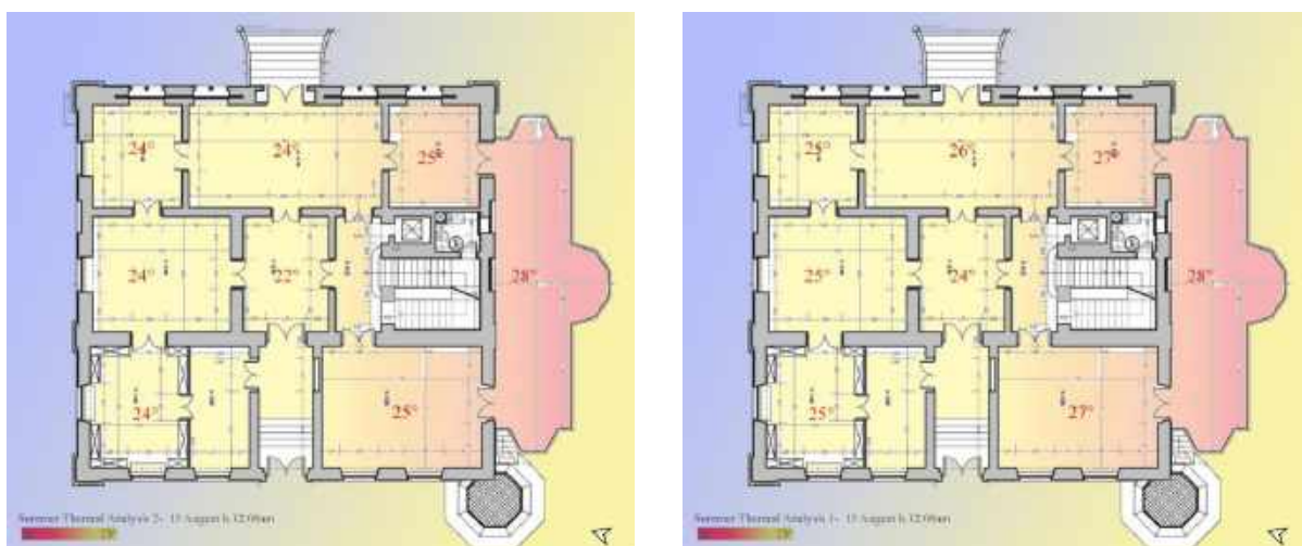
Fig. 9: CFD analysis in summer in two different condition (closed and open Windows)- 12 p.m - winter garden-Villino Favaloro.
