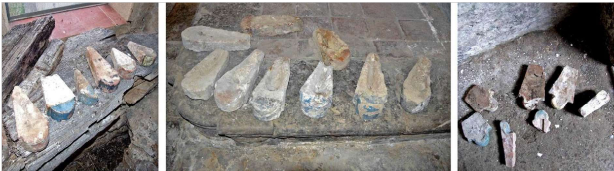
Fig. 3: Sicily, examples of wedge-shaped bricks used in the same spire with different tapering angles.
