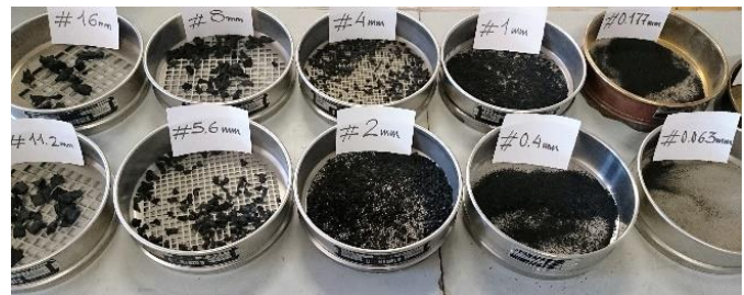
Fig. 16 Sieve analysis of the rubber from discarded truck-tires
