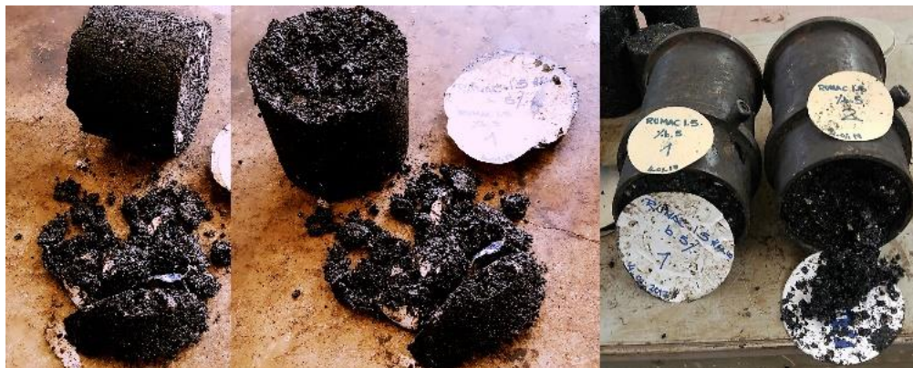
Fig. 5 Swelling effect on rubber-modified HMA samples of Ø150x120mm manufactured according Superpave SGC
