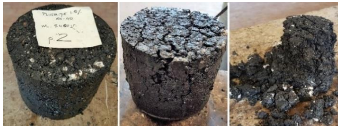
Fig. 7 Post-compaction deformation by rebound effect with rubber mixtures compacted with gyratory compactor
