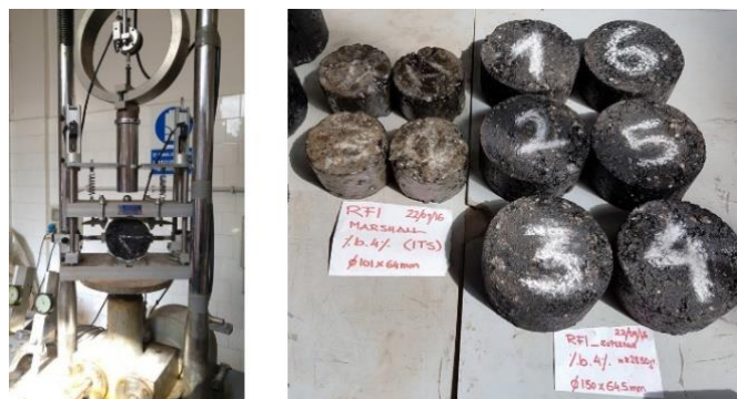
Figure 21. (a) IDT device, and (b) Marshall specimens for IDT and water sensitivity tests
