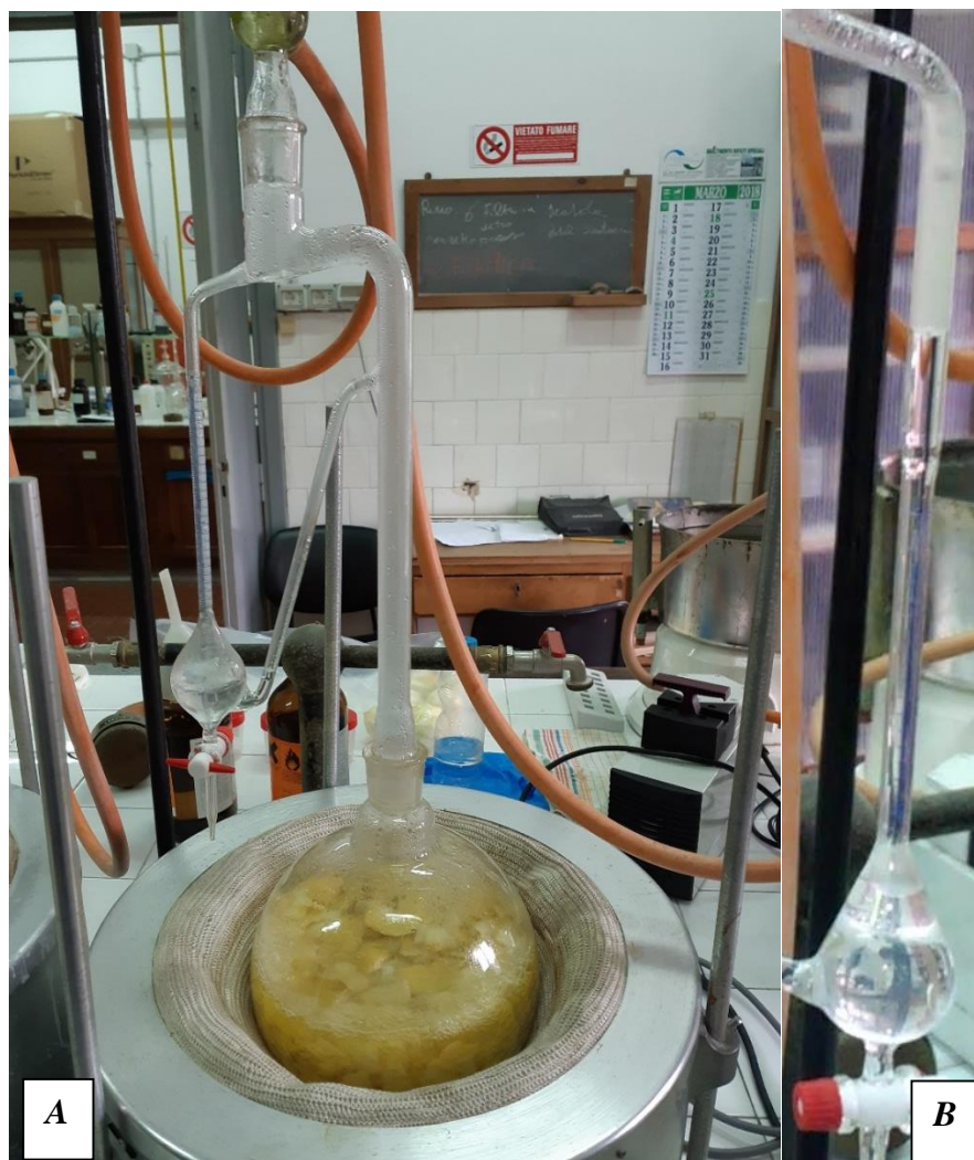
Figure 3_2. (A) EO extraction from lemon peels with Clevenger Apparatus. (B) Detail of lemon EO extracted.
