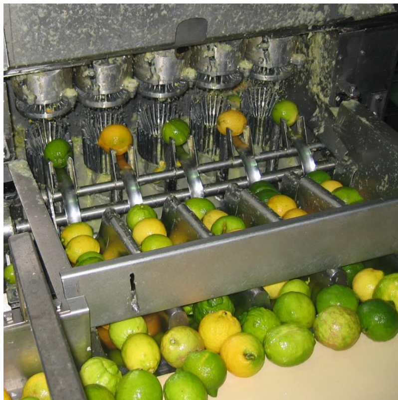
Figure 3_1. FMC juice extractor. Load of the calibrated fruits inside the cups.
