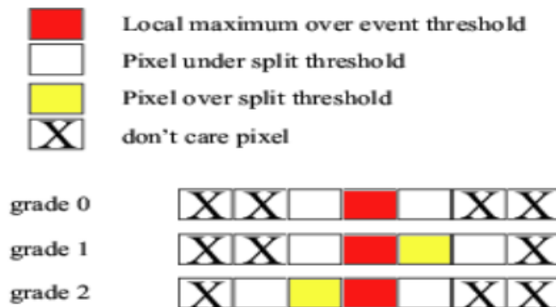
Figure 4.5: Definition of the XRT good grades for WT mode. The figure shows a 7 \times 1 matrix centred on the pixel containing the higher charge (local maximum, red) which is used to define the event grade, the pixels exceeds a defined threshold value (yellow) and the pixels with a charge under the threshold value (white). Figure from Capalbi et al. (2015).
