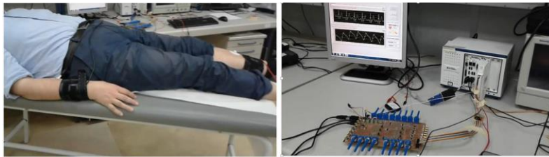
Fig. 2. Experimental setup and first measurements obtained on an intermediate PPG/ECG combo system composed by 3 synchronized PPG probes and 3 ECG leads.
