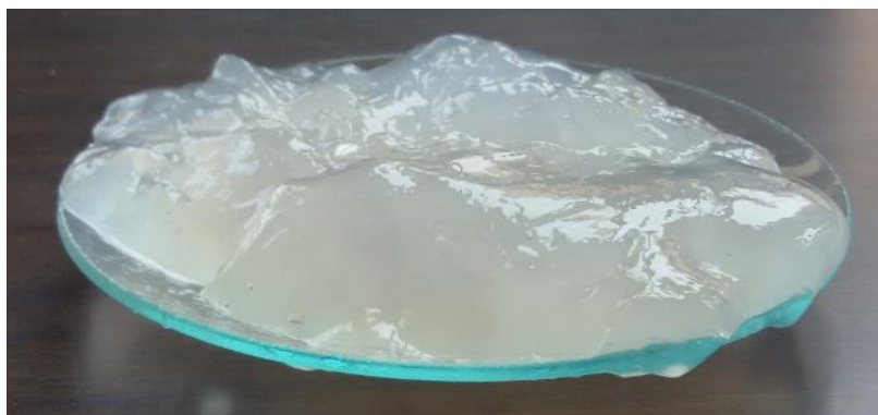
Figure 3.24 Hydrogel obtained with one cycle of freezing – thawin [12].
