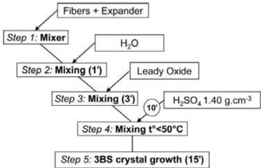
Figure 2.1 Preparation of 3BS pastes for negative plates [9].
