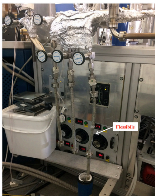
Fig. 1 – Flexibles connected to the UHV line of the Mass Spectrometer
