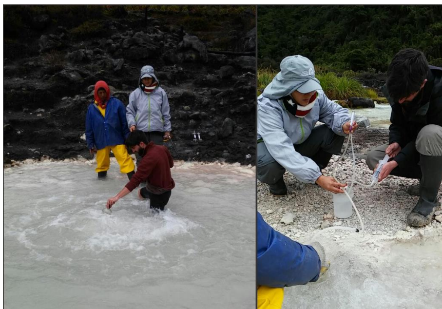
Figure 2.4: Sampling of dry gases from bubbling springs at San Juan de Purace (Colombia)
