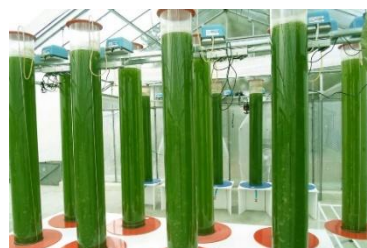
Figure 1.17: Microalgae cultivation in bubble column reactors at Sea & Sun Technology GmbH. https://www.abire.org/consortium/s
