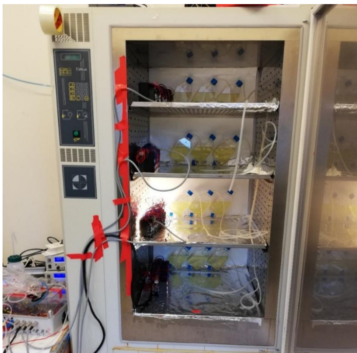
Figure 3.23: Culture system used for the experiment. The tissue flasks were placed in a cultivation chamber with regulated temperature. Each shelf contained a biological triplicate exposed to a different light condition. Led light source are showed.
