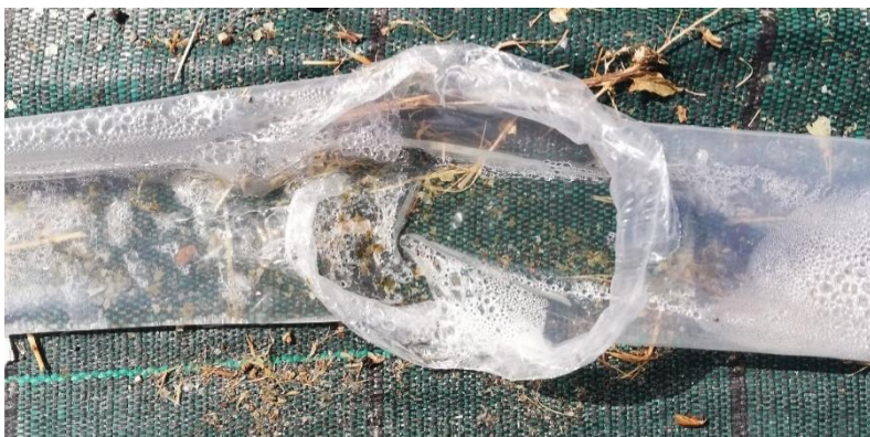
Figure 5.8: On the left the LDPE tube firstly employed is shown, while the mixed polyolefin tube successively employed is on the right
