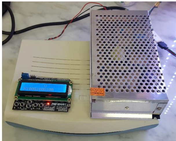
Figure 3.12: Final system supplied with an Arduino, the LED shield (inside the box), a led display with controller and a power pack.
