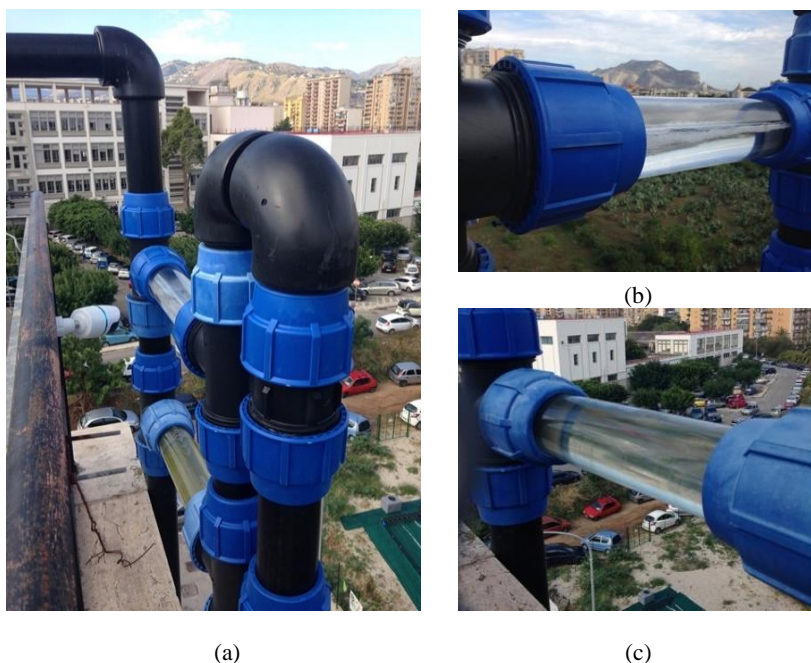
Figure 5.5: (a) Dual transparent degasser (b) full of air in the highest section and (c) of aqueous solution in the lower section.
