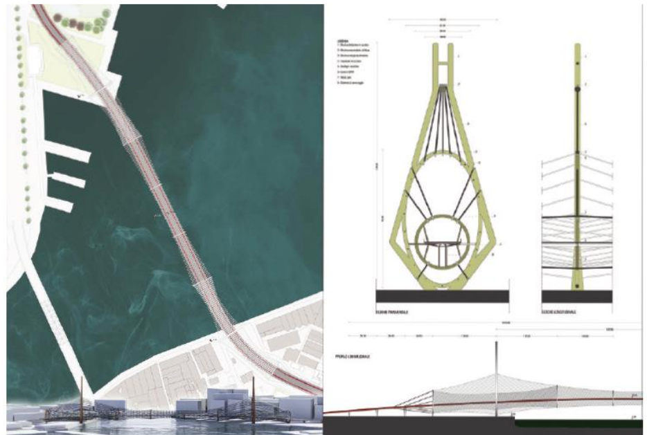
Fig. 14, 15 - Top: Plan of Busan with the new underground light-railway connecting the North Port peninsula with the nearby island of Yeongdo. Down: Plan and section of the Bridge of Peace in the Bay of Fusan-ko in Busan with its 140-metres steel tower (Graduation thesis of F. Settecasti).
