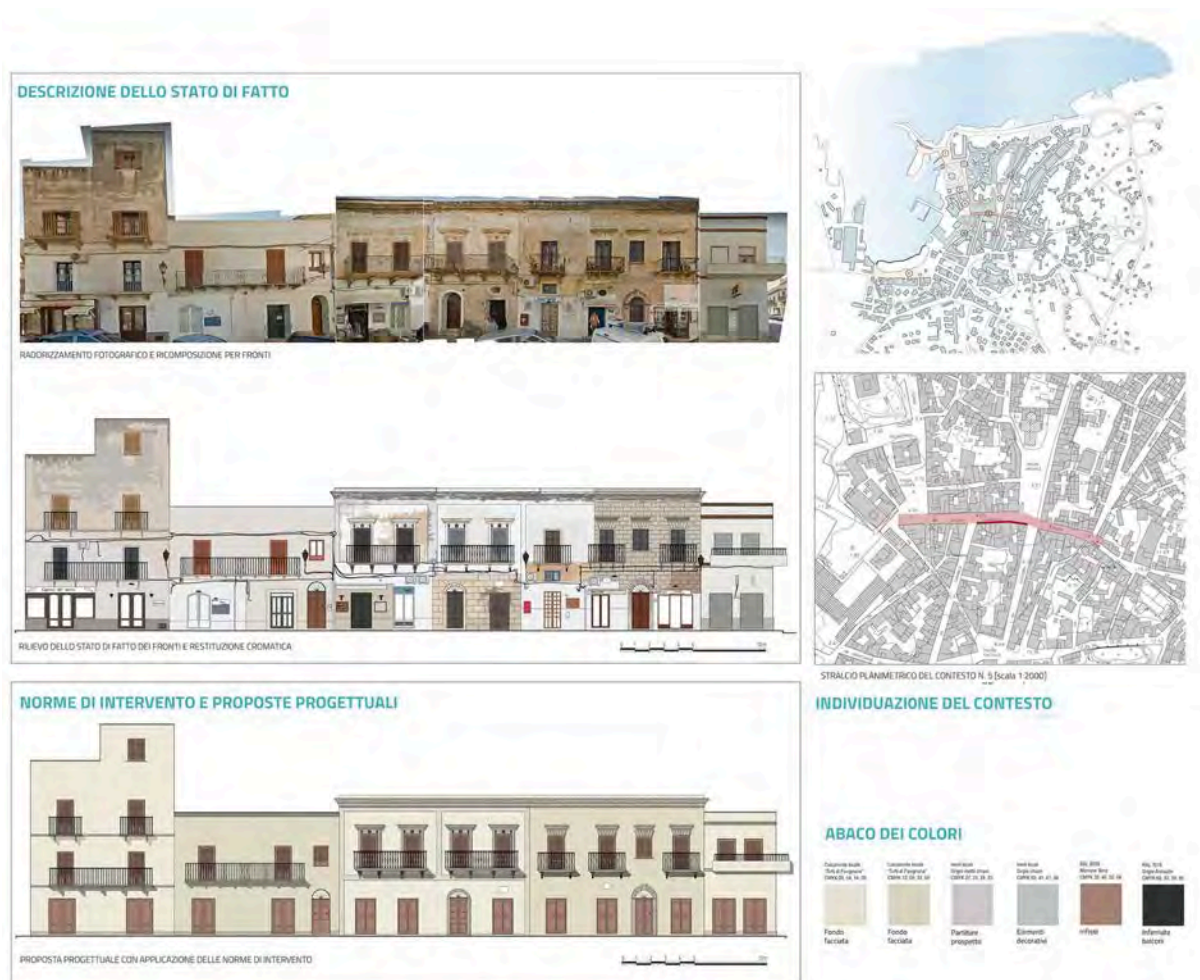
Fig. 20: Favignana Island, Vittorio Emanuele street. Analytical-proactive elaborations: analysis of the current state of the buildings, definition of the intervention rules, selection of the colour abacus, design simulation.
