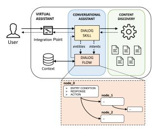
Fig. 2: Virtual assistant architecture. Users interact with the system through an *integration point*, which forwards the requests to the *dialog skill* in order to recognize *intents* and *entities*. Optionally, the *content discovery* module is called to extract relevant information from unstructured documents. The *dialog flow* produces the correct answer, which is later shown to the user through the same *integration point*.
