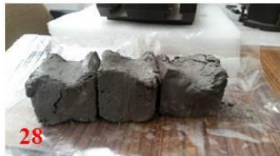
Fig.5. Specimens cured at -20°C that did not harden. From top: 1, 7, and 28 days of curing.
