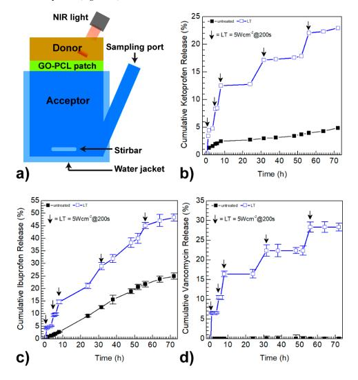
**Figure 4.** Drug release study of the loaded GO–PCL patches in PBS pH 7.4 after five cycles of near infrared (NIR) photo stimulation: each arrow indicates the exposure to an 810 nm laser diode for 200 s and a power density of 5 Wcm<sup>-2</sup>.
