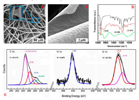
**Figure 1.** SEM analysis (**a–a**') of the GO–PCL sample. Fourier transform infrared (FTIR) spectra of PCL (black), GO–PCL (red), and GO (green) in the region within 1800–800 cm<sup>-1</sup> (**b**). X-ray photoelectron spectroscopy (XPS) spectrum of GO–PCL: experimental spectrum (black), composite spectrum (grey), and deconvolution peaks are showed as colored curves (**c**).
