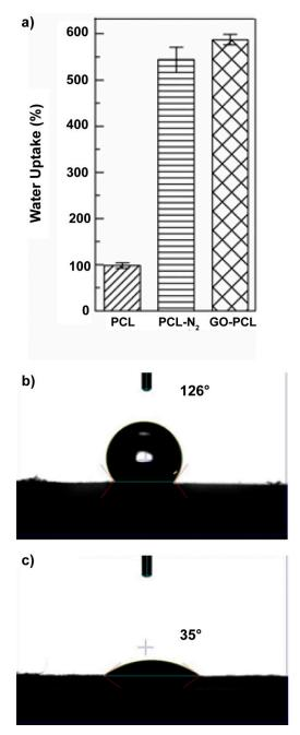
Figure 2. Water uptake (a) and water contact angle measurements for the virgin PCL (b) and GOPCL patches (c).
