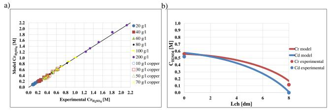
**Figure 1.1.** a) Batch operation: calculated retentate sulfuric acid concentration versus experimental retentate sulfuric acid concentration for different initial sulfuric acid concentrations (filled marker) and for a constant initial sulfuric acid concentration of 60 g/l for different initial copper concentration. b) Continuous operation: calculated and experimental sulfuric acid concentrations along the retentate (r) and diffusate (d) channels.
