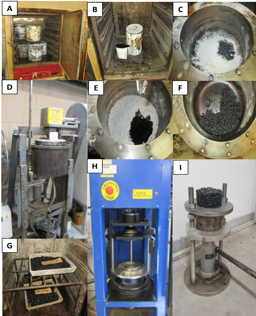
Figure 5.5: Steps of samples manufacturing.
