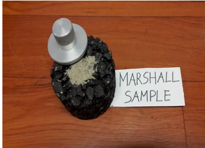
Figure 3.4: Miniaturised MTD (Marshall sample, V= 4500 \text{ mm}^3 , Praticò, Noto and Astolfi, 2017)
