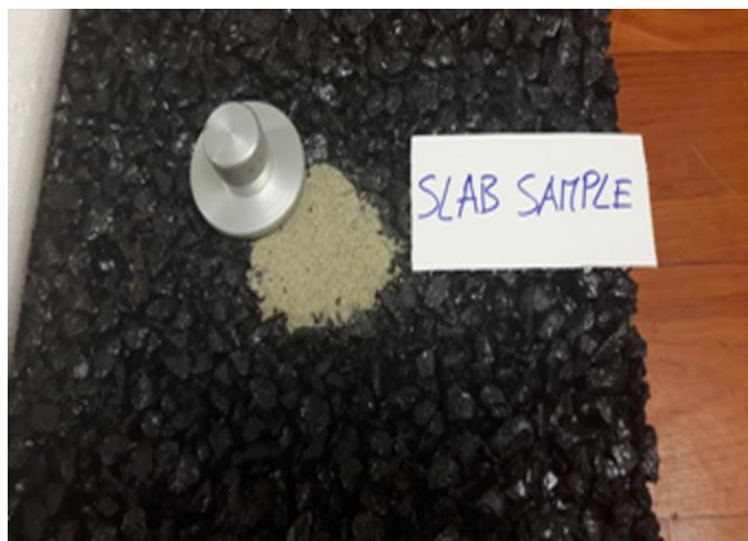
Figure 3.6: MTD ("pavement" sample, current method with V= 25000 \text{ mm}^3 , Praticò, Noto and Astolfi, 2017)
