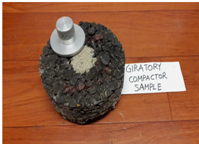
Figure 3.5: Miniaturised MTD (Giratory sample, V= 4500 \text{ mm}^3 , Praticò, Noto and Astolfi, 2017)
