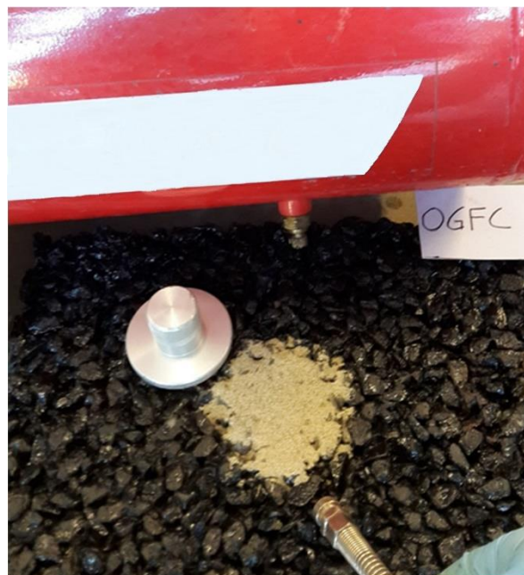
Figure 3.9: Cleaning of the pavement between two successive tests on the same point of the surface (Praticò, Noto and Astolfi, 2017).
