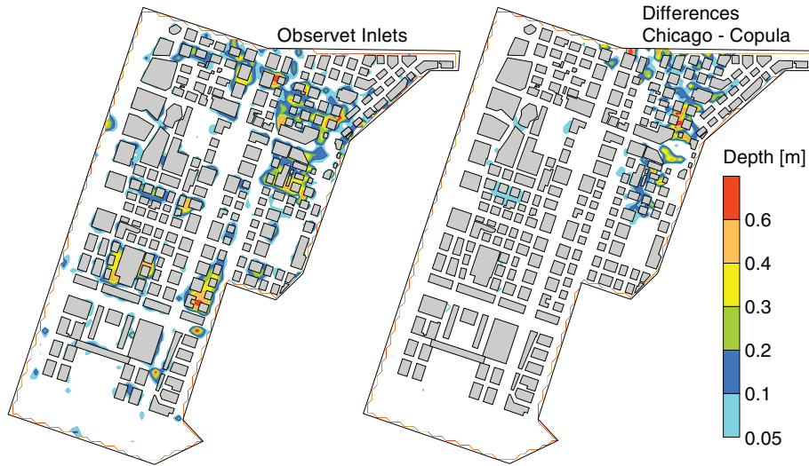
Figure 9 Maps of maximum water depth obtained for the copula-based hyetograph at the 10-year return period. The map related to the observed inlet conditions is plotted together with the map of differences between the maximum water depth obtained for the Chicago and copula-based hyetographs.
