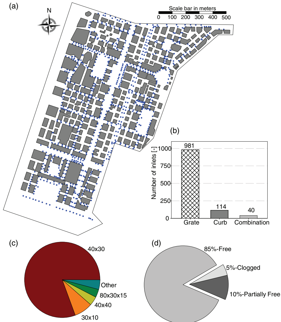
Figure 2 Location (a), type (b), geometry – in centimetres – (c) and clogging condition (d) of storm water inlets in the Foce subcatchment.
