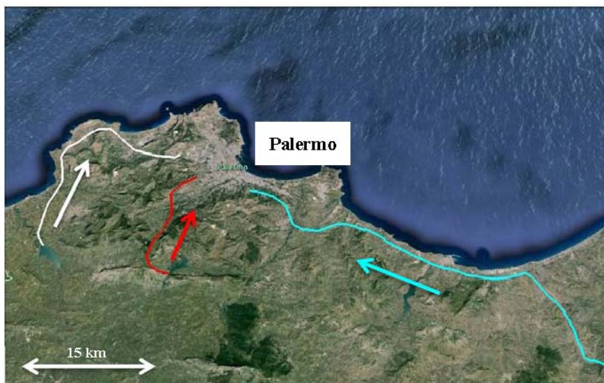
Figure 1. The water supply scheme in Palermo: the Jato system (in white); the Gabriele System (in red) and the Scillato System (in cyan).
