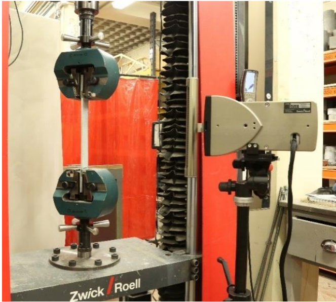
Figure 2. Test setup of composite strips
