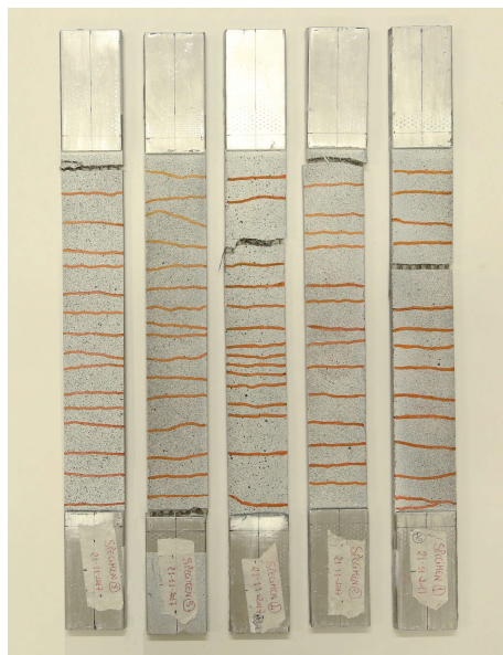
Figure 4.28 Two-layer reinforced BFRCM specimens after testing
