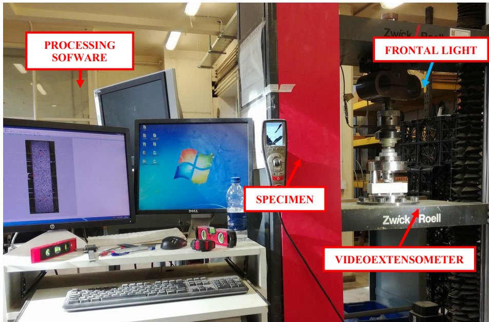
Figure 3.15 Three point bending tests: test setup
