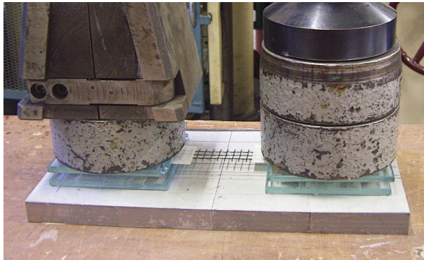
Figure 3.9 Preparation of basalt fabric strips
