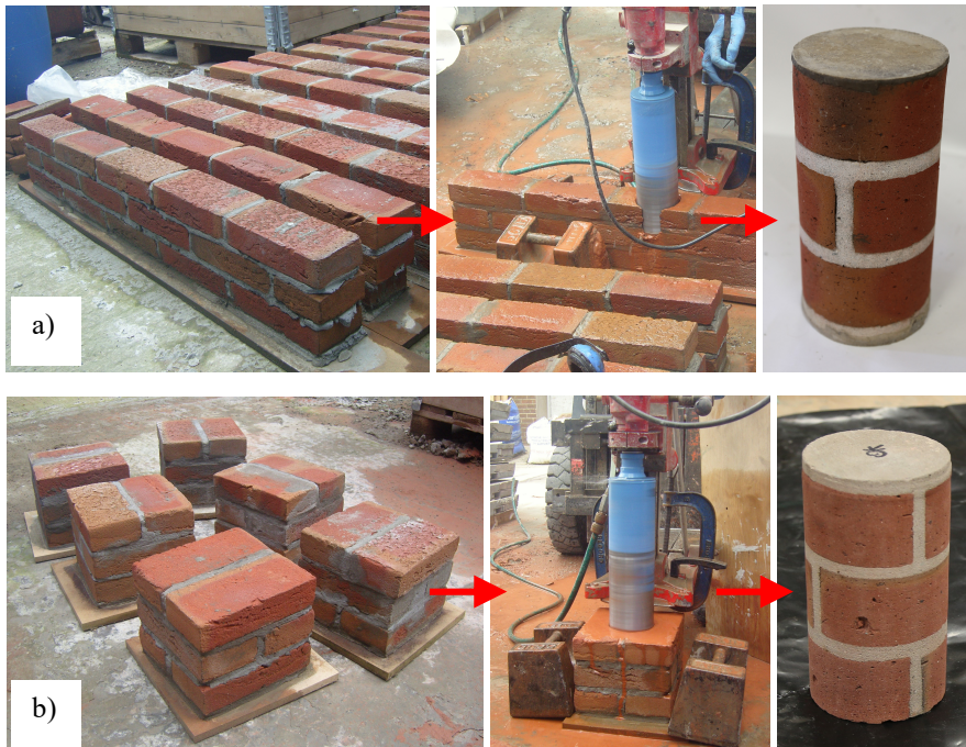
Figure 3.26 Brick assembly schemes for preparing cylinders: a) Scheme I (wall); b) Scheme II (column)
