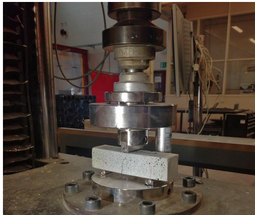
Figure 3.16 Three point bending tests: specimen during testing
