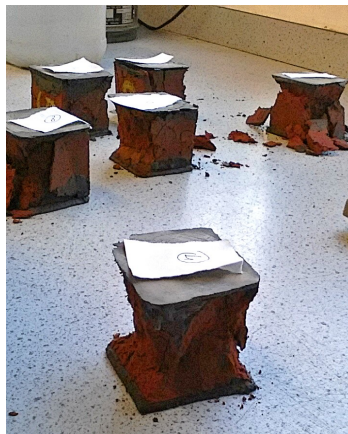
Figure 4.1 Brick cubes after compressive tests
