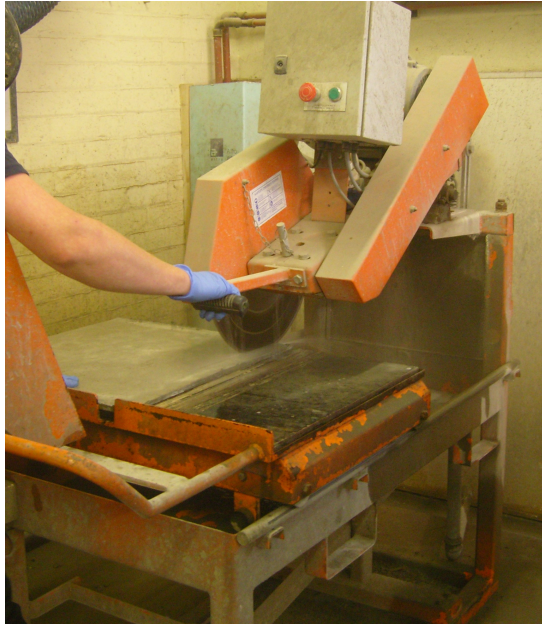
Figure 3.18 Cutting of the BFRCM slab
