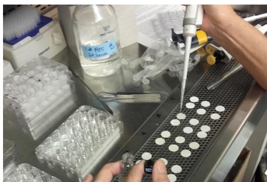
Figure 53 - Preparation of the samples: soaking filter paper disks
