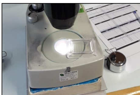
Figure 92 - Detail of visual assessment: counting plate under the microscope
