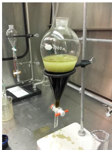
Figure 45 - Separatory funnel during the partitioning process. Detail of two separated solvents of different density
