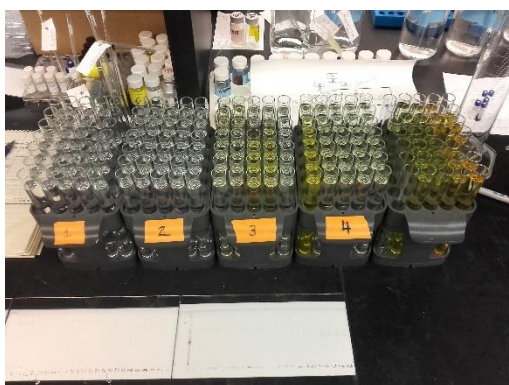
Figure 60 - racks of 22 mL glass tubes filled with fractions recovered after flash chromatography
