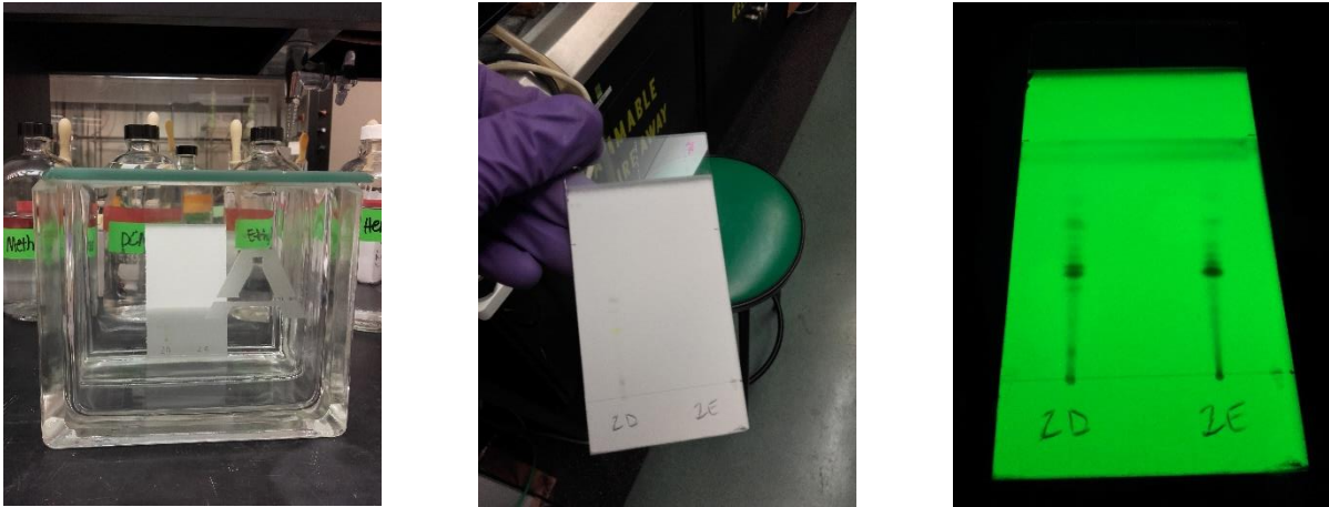
Figure 48 - (left to right) Thin-layer chromatography; TLC plate after the elution; TLC plate under UV light.
