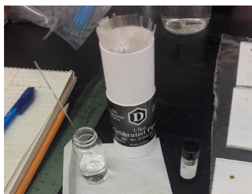
Figure 71 - Preparation of the samples: spotting crude extracts on TLC plates
