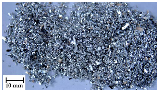
Figure 3.12. AZ31B milled chip used for the experimental campaigns.
