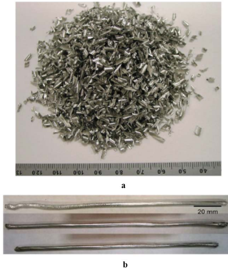
Figure 3.2. (a) AA6061 chips and (b) wires (source [94]).
