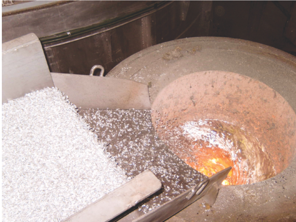
Figure 2.4. LOTUSS vortex furnace (Source: Pyrotek).
