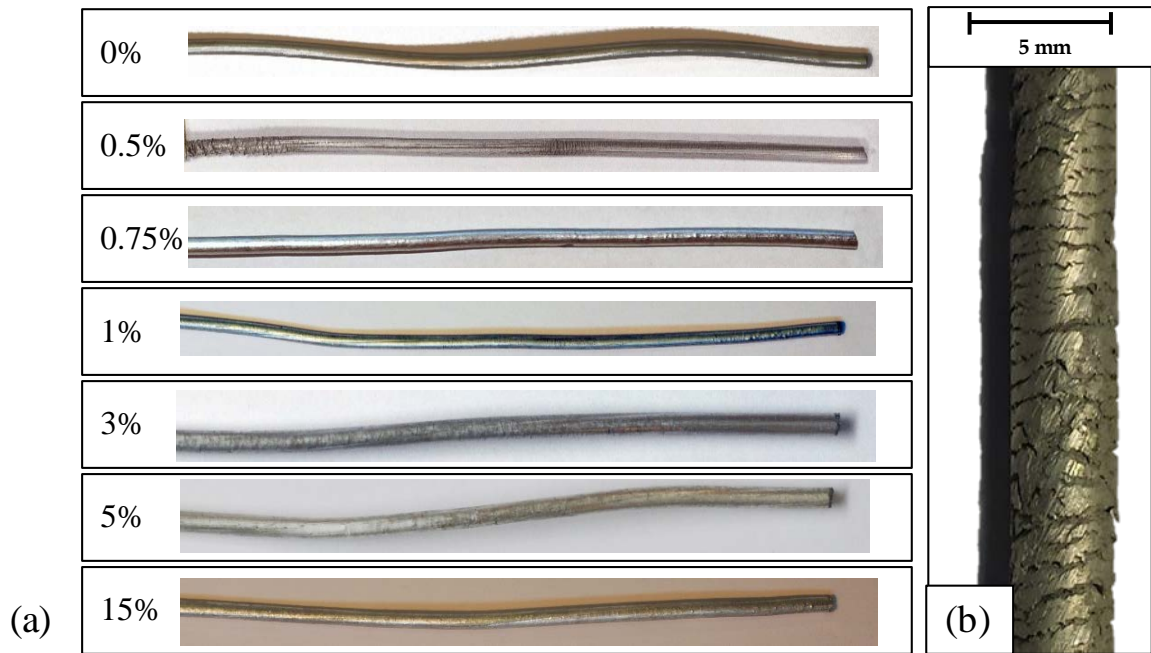
Figure 3.38. (a) Extruded wire with varying the added volumetric percentage of SiC powder and (b) detail of the cracks for the p=15\% case study.
