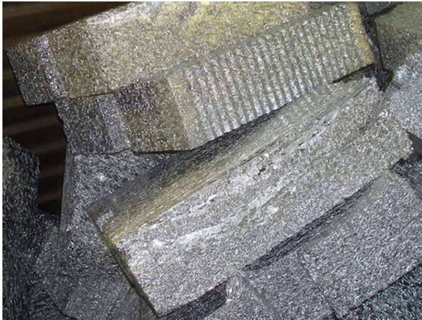
Figure 2.3. Metal chips briquettes (Source: Pyrotek).
