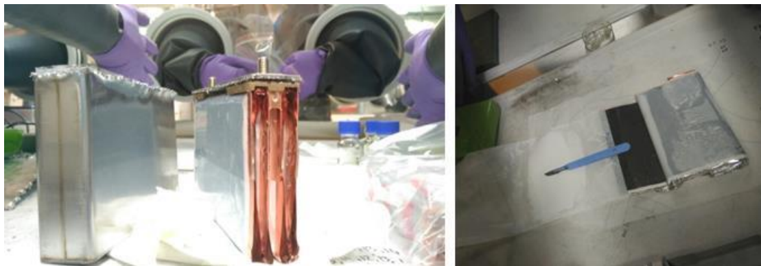
Figure 44. Left, components of a fresh LMO-NMC/graphite cell after opening and removing the cell casing in a glove box; right, unfolding of one of the two prismatic jelly rolls [118].
