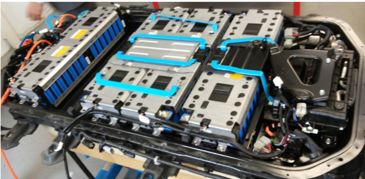
Figure 13. Mitsubishi Outlander PHEV battery pack.
