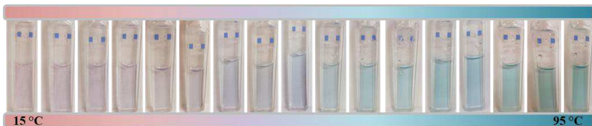
Figure 47 - Colour shades for the system [N_{1.13GA.8}]Br/Co(NTf_2)_2/[N_{2.22.4}][NTf_2] .
