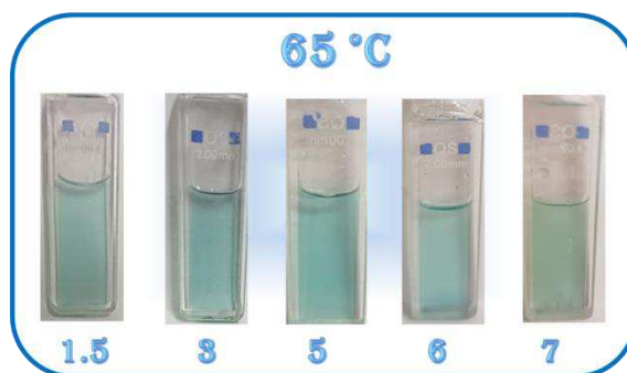
Figure 36 - Solution of [\text{N}_{1.12}\text{GA}_8]\text{Br}/\text{Co}(\text{NTf}_2)_2/[\text{N}_{2.224}][\text{NTf}_2] at 65 °C, varying the ligand/metal ratio from 1.5:1 to 7:1.
