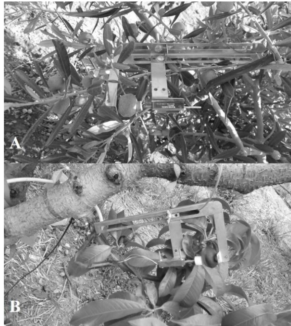
Figure 2.5. Fruit gauge mounted on an olive drupe at its growth stage III (A) and on a nectarine fruit at its growth stage I (B).
