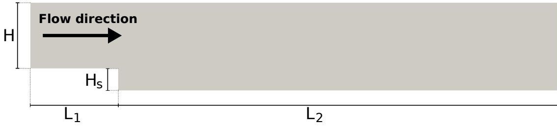
Figure 7.8: Benchmark test case - Sec. 7.4.5. Channel geometry. H = 10 \text{ mm} , H_s = 7.5 \text{ mm} , L_1 = 10 \text{ mm} , L_2 = 50 \text{ mm} .
