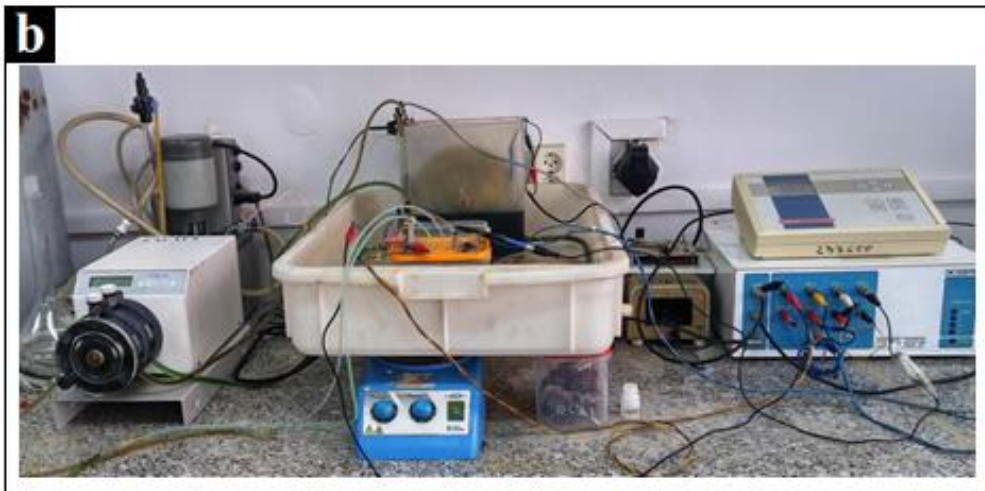
Figure 4.4.1.1 a) Schematic representation and b) photo of the experimental apparatus for dismantling/leaching of WPCB and simultaneous copper recovery. From figure a): 1- Leaching reactor, 2- electrochemical cell for copper recovery, 3- leach solution container, 4- peristaltic pump, A- anode, C- cathode
