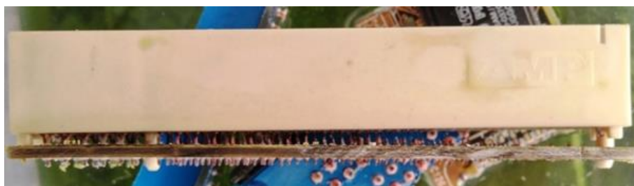
Figure 4.2.2.1 Photo of a PCI slot after leaching without air blowing in \text{H}_2\text{SO}_4\text{-CuSO}_4\text{-NaCl} solution
