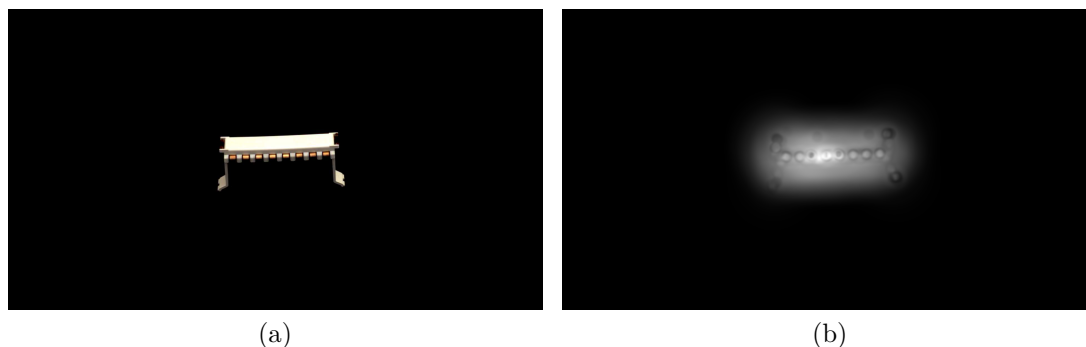
Figure 3.7: (a) An image from the OPED and (b) its saliency map calculated in L^*u^*v^* space using the SURF keypoint detector, multi-scale map generation, polynomial fusion and center bias weighting.
