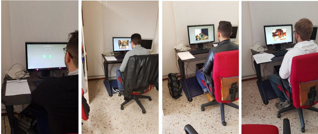
Figure 3.15: Images taken during the eye-tracking session: starting from the calibration (the far-left image) the eye-tracker records the eye movements, the saccadic movements and the scanpaths.
