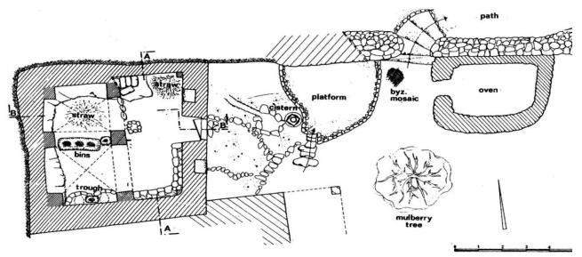
Figure 1: The plan of a typical traditional house, including the external yard, Palestine (Hirschfeld, 1995).
