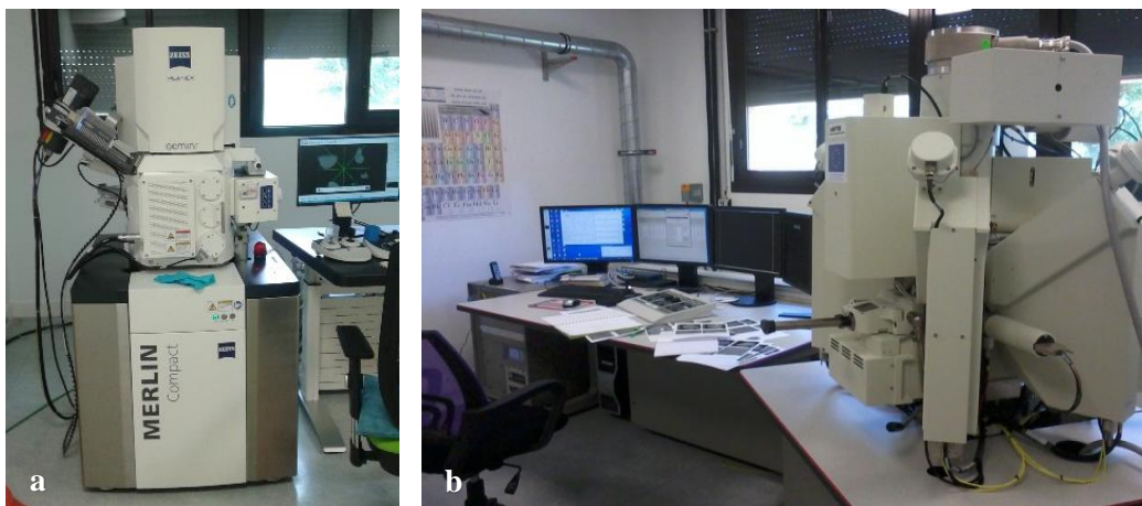
Fig. 3.2 - a) Scanning electron microscope and b) electron microprobe at the ISTO-CNRS used for observations and analyses of the samples.
