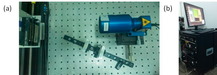
Fig. 2. Set-up for the laser ultrasound experiments (a) and the laser controller station (b).
