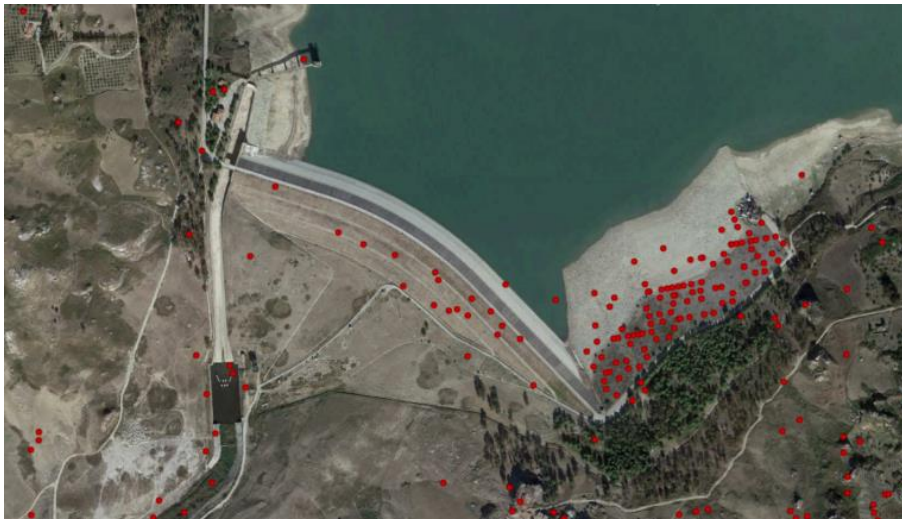
Figure 4. 16 Selected PS with high coherence ( > 0.7 ) located over the dam
