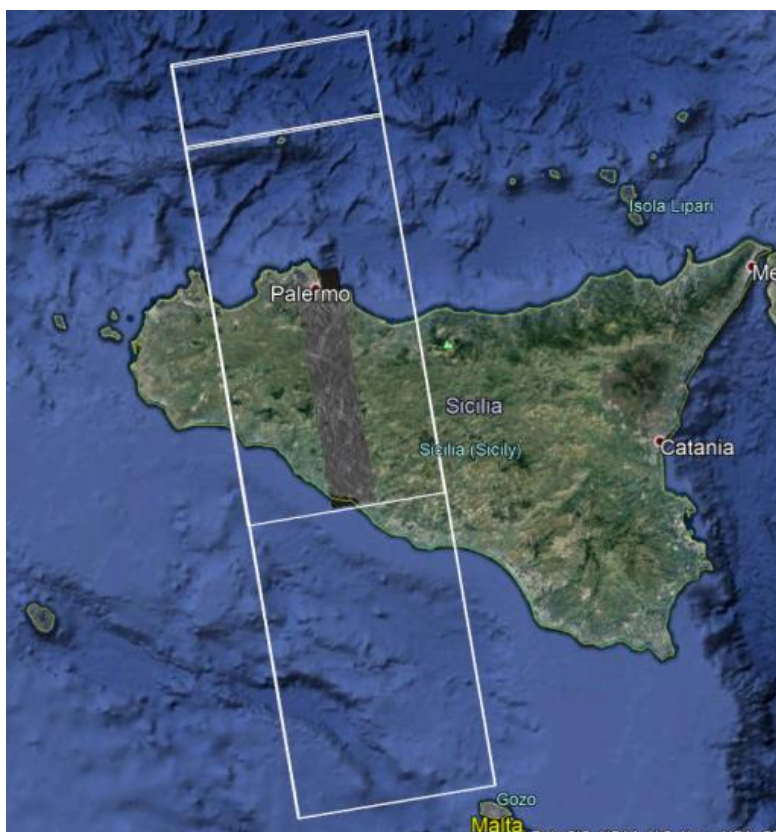
Figure 2. 8 View of ascending track 117 (white boxes) from IW2 of the S-1A dataset covering the study area in Sicily (Italy) (image available from Google Earth Professional).
