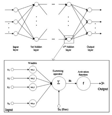
Fig. 5. Pictorial representation of the multilayer feedforward neural network
