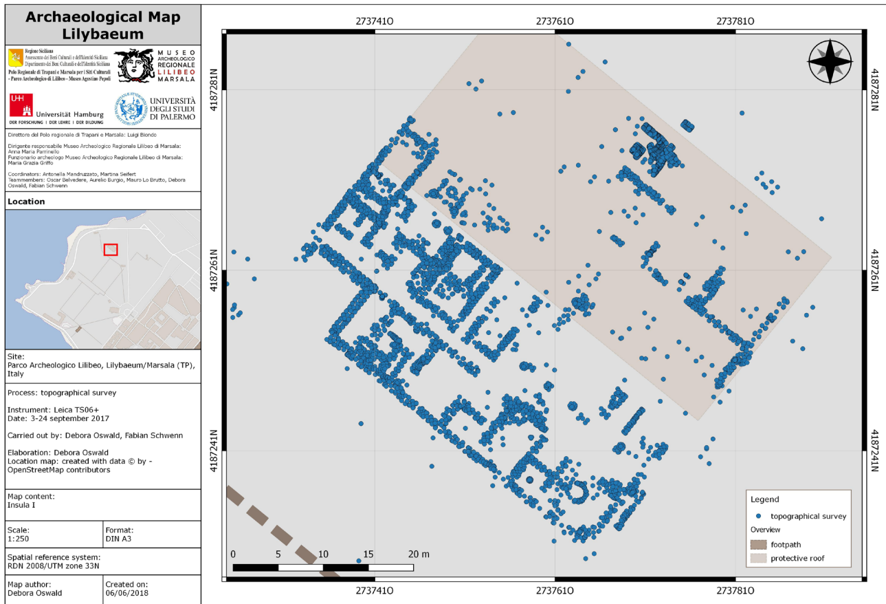
Fig. 3 Visualised measurements of the topographical survey of Insula I in 2017.
